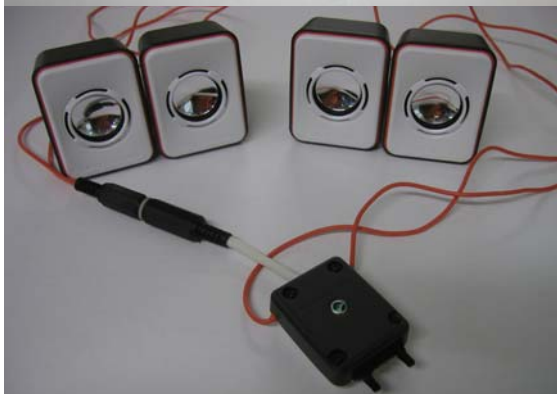
Fig 8: Modified external speaker set including a second pair of speakers connected in parallel to the original pair.
