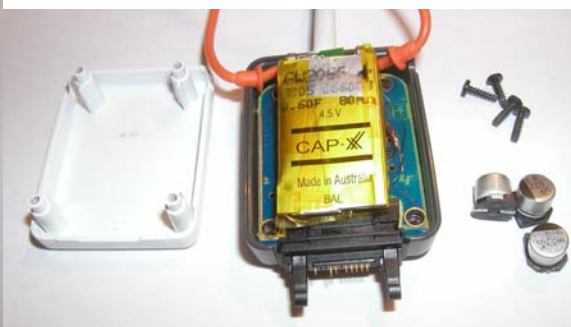
Fig 7: External audio amplifier, powered from the phone, modified to include a supercapacitor
