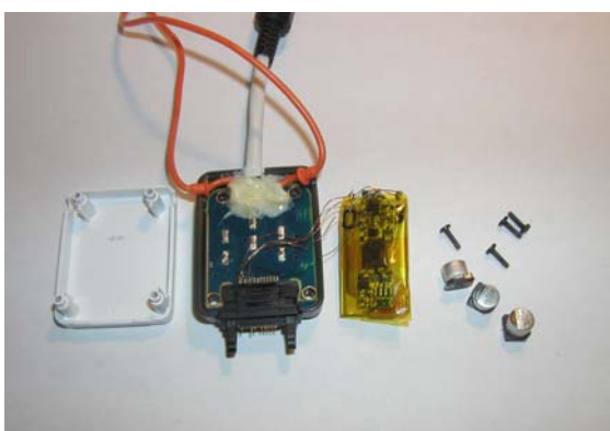
Fig 7: External audio amplifier, powered from the phone, modified to include a supercapacitor
