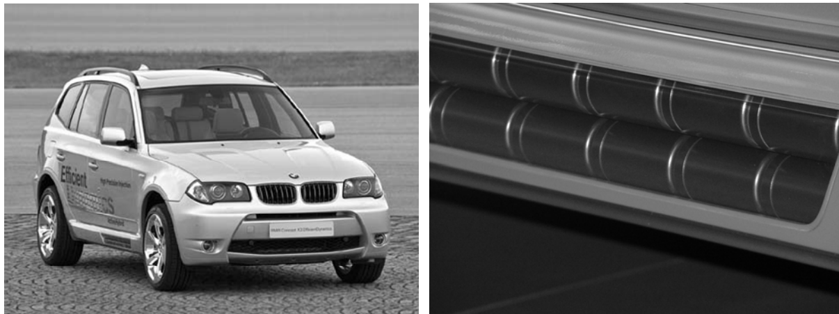
Figure 8: BMW X3 with 190kJ ultracapacitor tube modules in the door sills
