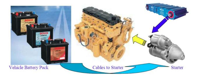
The most important aspect of the illustration above is cable length and termination guality. To appreciate this fact consider the resistance of copper cable in Ohms/foot:
