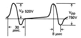
The Vrms voltage derived from the peak voltage shall always be less than the nominal AC voltage rating of the capacitor.
